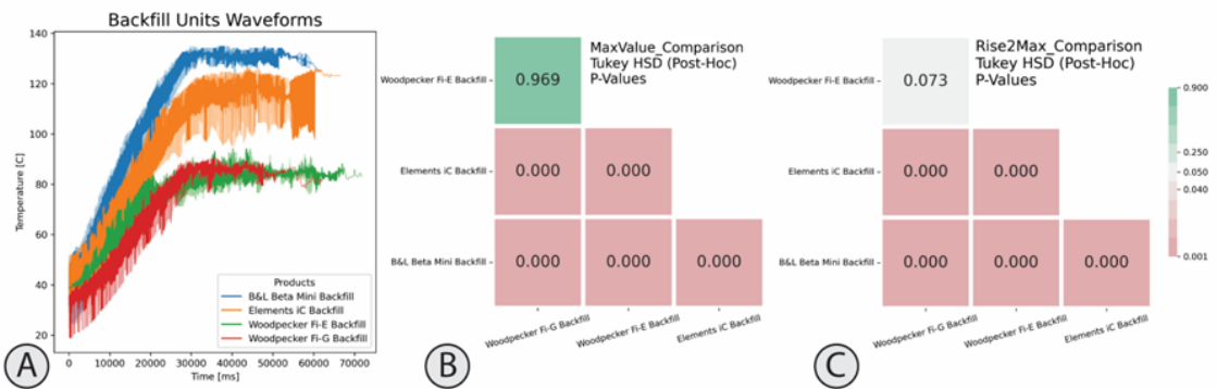
Figure 2. Results from the Backfill unit testing: (A) median plot for each product group in bold with 95% confidence interval in background shading, (B) Tukey HSD test results for the max value test on temperature, (C) Tukey HSD test results rate of temperature change when heating.
