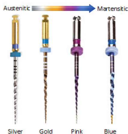
Figure 1. Diagram illustrating the heat-treatment color spectrum of files, ranging from more austenitic to more martensitic.
