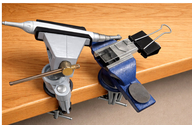
Figure 3. Intra-experiment image of bench vise set-up with endo handpiece and metal block (Images were captured with an iPhone 15 Pro (Apple Inc., Cupertino, CA, USA) using the native camera application).
