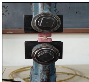
Figure 5. Specimen mounted on Universal Testing Machine
