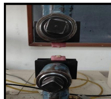
Figure 6. Measurement of shear bond strength
